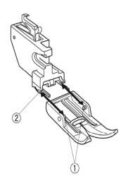
To install, simply remove the exiting foot from your AcuFeed Holder by pulling the foot towards you.
